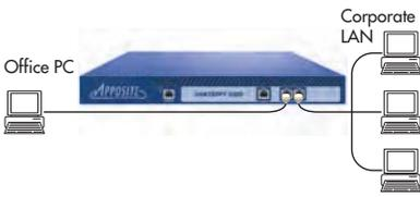
Alternatively, the Linktropy device can be installed between the user's office PC and the corporate LAN. The office PC will then act as if it were located at a remote office, with full access to all corporate applications without the need for a separate lab or any special set-up.
