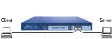
To test a single application on an isolated network, simply plug in a client (or a network of clients) into one emulation port of the Linktropy unit, plug in the server (or a network of servers) into the other emulation port, and configure the link bandwidth, latency, loss rate and any other impairments through the browser-based interface.
